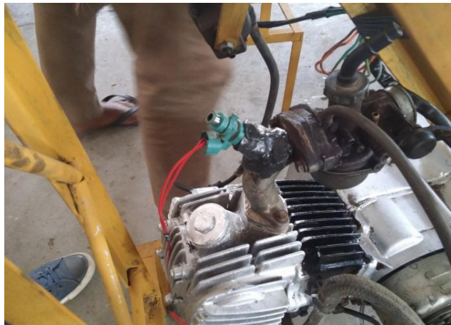
fig 3.6 installation of ethanol fuel injector
