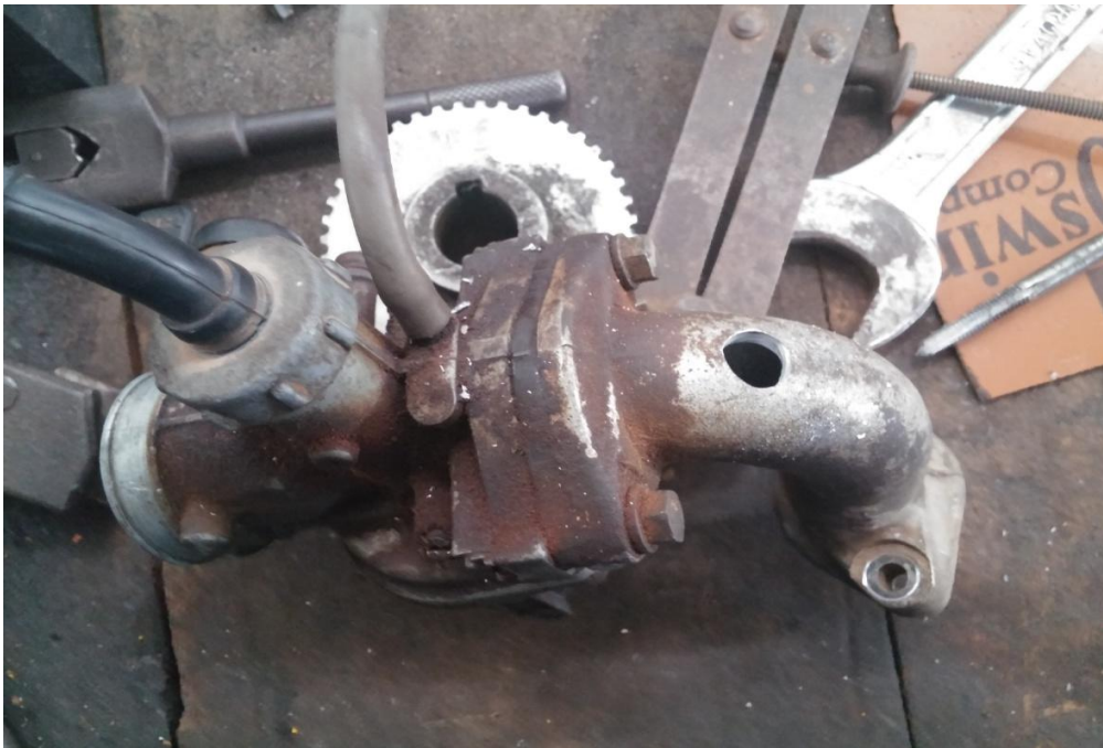
Fig3.2 inlet manifold after drilling
