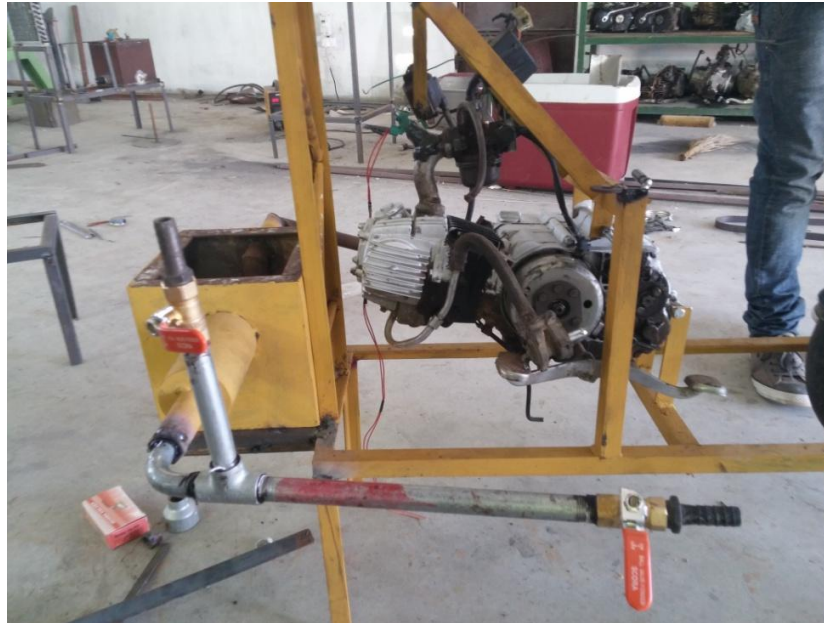
fig 3.8 EGR system installed on the frame
